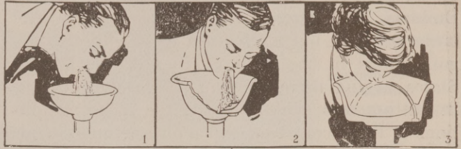
Vertical Stream Bubbler Condemned Everywhere Camouflaged Vertical Stream. Rainbow Stream, Hose like; difficult to drink from.
